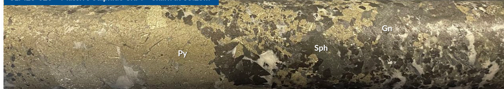
SLM23-020 – Massive Sulphide CRM + Skarn at 35.25m
