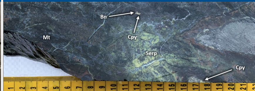
LAV22-006- Magnetite(Mt)-Chalcopyrite(Cpy)-Pyrrhotite(Po) Skarn at 167.10m
