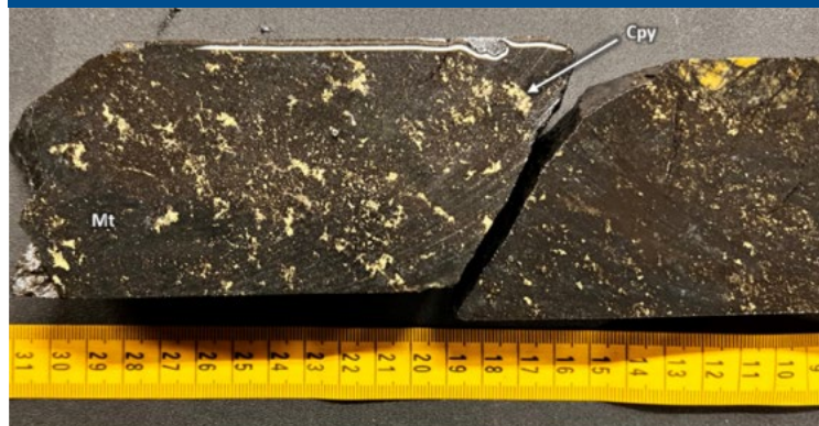
LAV22-001 - Magnetite(Mt)-Chalcopyrite(Cpy)-Pyrrhotite(Po) Skarn at 78.45m
