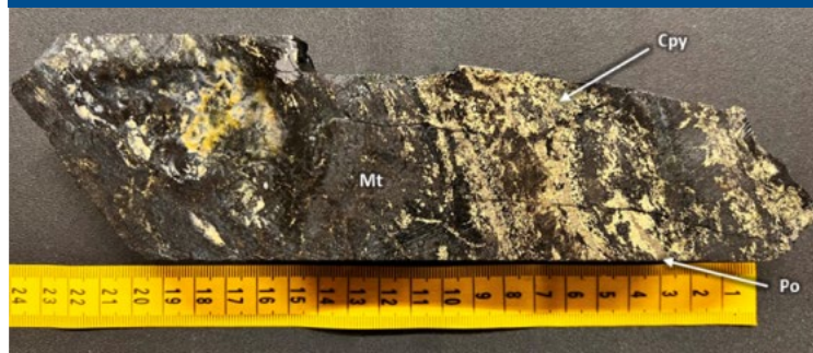
LAV22-001 - Magnetite(Mt)-Chalcopyrite(Cpy)-Pyrrhotite(Po) Skarn at 78.45m
