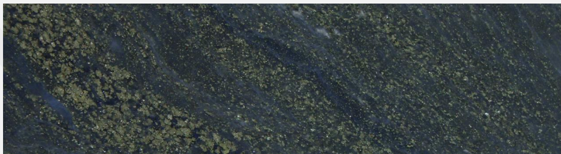
Silicified sericite schist with abundant chalcopyrite
