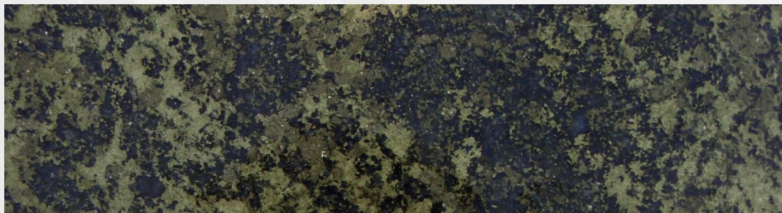
Sericitic limonite with abundant chalcopyrite +/- covellite
